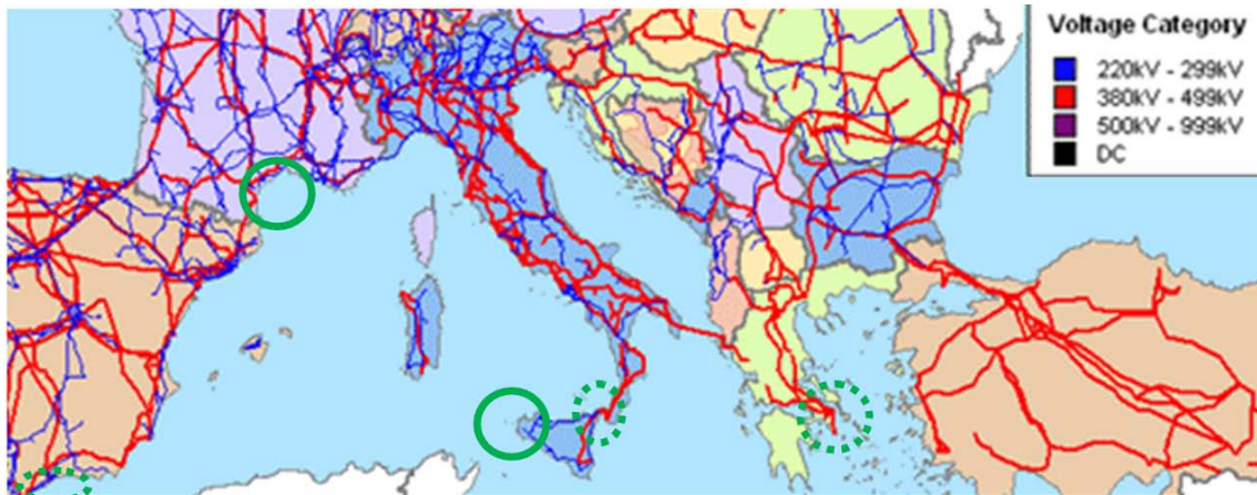
Figure 87: Mediterranean and Black Seas: Electrical Grid Infrastructure (Solid Circles: Wind + Wave Sites, Dotted Circles: Wind + Tidal Sites)
