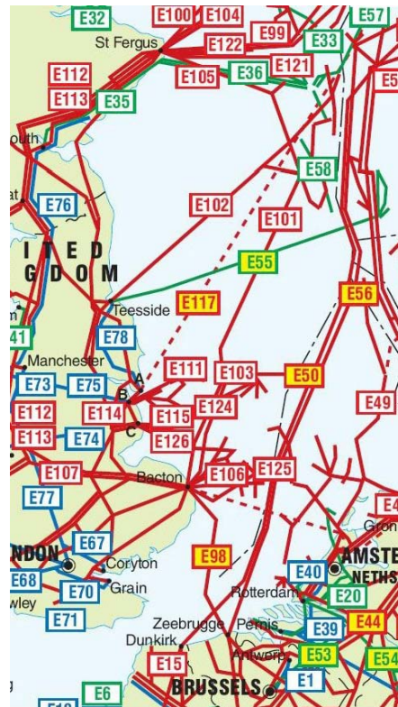
Figure 27: North Sea Oil Pipelines 58
